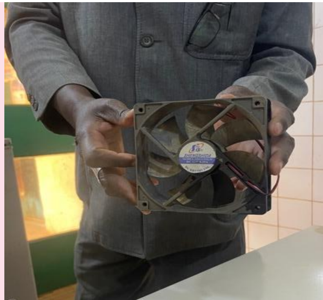
A PMT in Tahoua shows that fridge fans are parts that break frequently. Photo: MOMENTUM Routine Immunization Transformation and Equity
